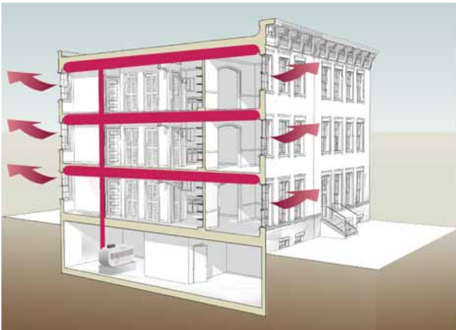
Leaky, poorly insulated envelope = Larger heating & cooling loads
